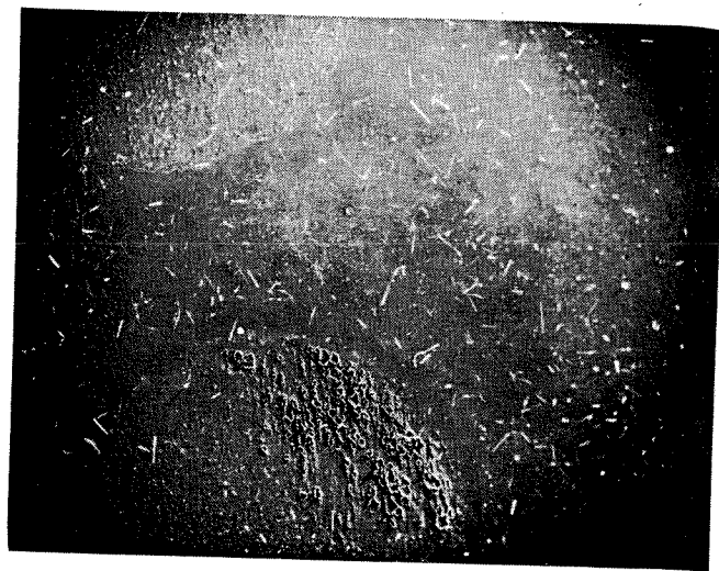
Fig. 7. Whisker growths on tin in contact with glass and with iron—Original magnification 24X.
